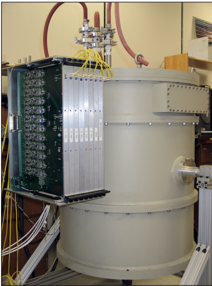
Figure 2.15 AzTEC cryostat and readout electronics in the UMass Amherst Cryogenic Device Laboratory 9 .
